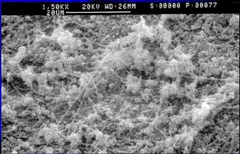
The SEM image shows a dense, irregular layer of material (fouling) on a surface. The top of the image contains technical data: 1.50KV 20KV WD:26MM S:00000 P:00077.
